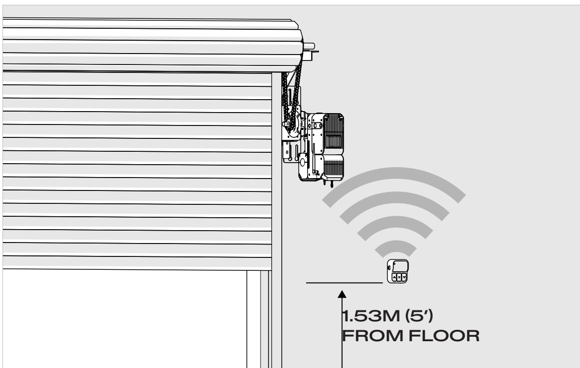
Typical setup with wireless console connection
