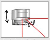
Adjust the tilt angle of the detection field witht the hex key if necessary.
