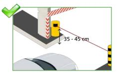
Install the sensor at a mounting height of 35 - 45 cm. If the barrier is only used by trucks, the mouting height can be increased.
