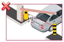
If the reference beam is too low or too high, vehicle collision with the boom cannot be excluded.
