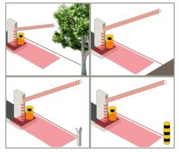
If the safety field is the only protection against collision with the boom, the safety field of the sensor must be situated right under the boom.
