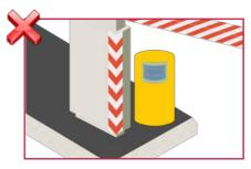
Do not cover the front face of the sensor with glass or plastic.
