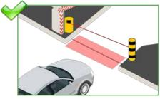
When using the safety, place the sensor just behind the barrier. This way the safety field protects the area around the boom.
