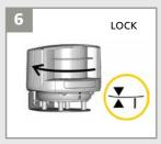
Turn the sensor until the two triangles are face to face.
