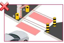
When using the safety, never place the sensor before the barrier (B) or more than 40 cm after the boom (A).
