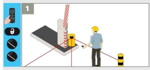
Activate the visible laser beams by remote control to position the sensor correctly.
