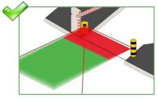
Make sure to place the detection field parallel to the boom.
