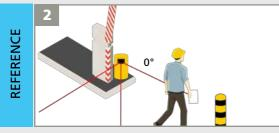
Use a white paper to verify the position of the 0° laser beam. The reference point can be adjusted on any object at the end of the boom or farther away. Its surface should be +/- 10 cm and it must be firmly fixed.
