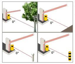
The sensor and detection field position are very important for the good functioning of the barrier.
