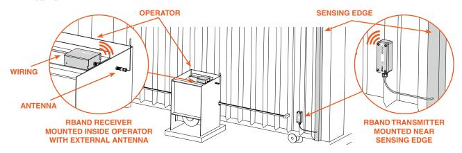
**IMAGE 1. RBand Transmitter Installation with Gate Edge**
