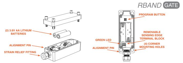
Note: RBand 10K Gate Edge Receiver is compatible with up to 3 RBand Transmitters on 2 channels (6 total).
