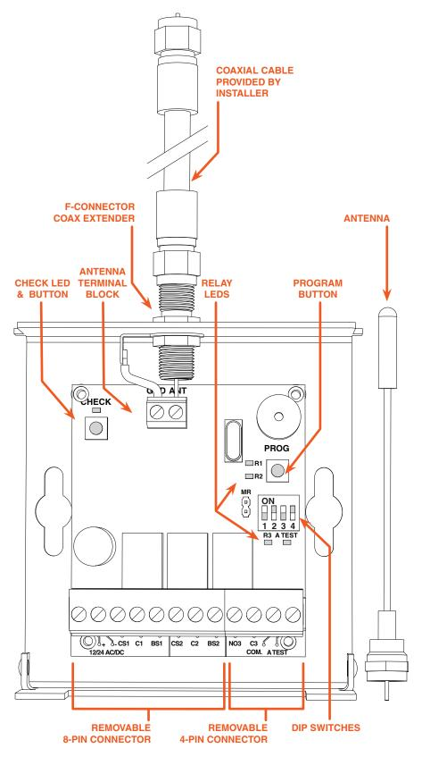
**IMAGE 2. RBAND GATE EDGE RECEIVER PCB & CONNECTIONS**
