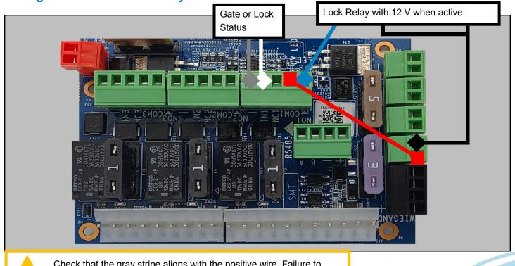
Check that the gray stripe aligns with the positive wire. Failure to use a diode with the lock voids the warranty.
